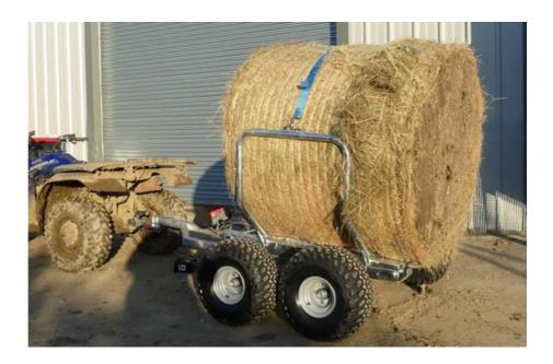
5. As the bale comes "over centre" press the locking catch rearwards again, and keep winding in the electric lift until the cradle is fully resting on the frame. Release the catch and ensure ensure the locking catch locks the bale securely into place.
