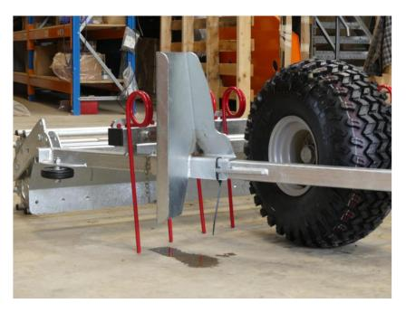
2. With the machine in transport mode remove steel pin and turn the blade to a 90-degree angle (see below) making sure the pin holes are aligned. The perimeter blade can also be used on the left-hand side of the machine.
