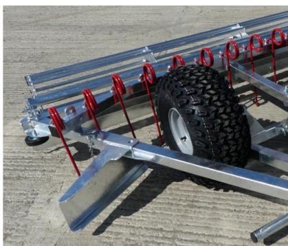
3. Slide the pin back into place, ensuring the blade is secure.
