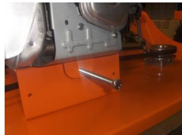
8. Tighten two M8 bolts in-front of engine using 13mm spanner
