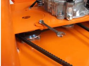
2. Loosen belt tension bolt behind engine with 17mm spanner anti-clockwise
