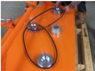
5. Pull belts from between pulleys 2 and 3 and place over engine pulley on highest groove
